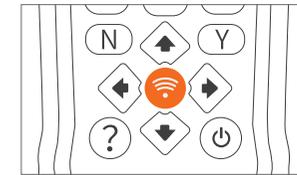
6. Through the up, down, left and right buttons, you can select the sensors on the four tires of the vehicle, and click the RF transmission button to activate them respectively.
